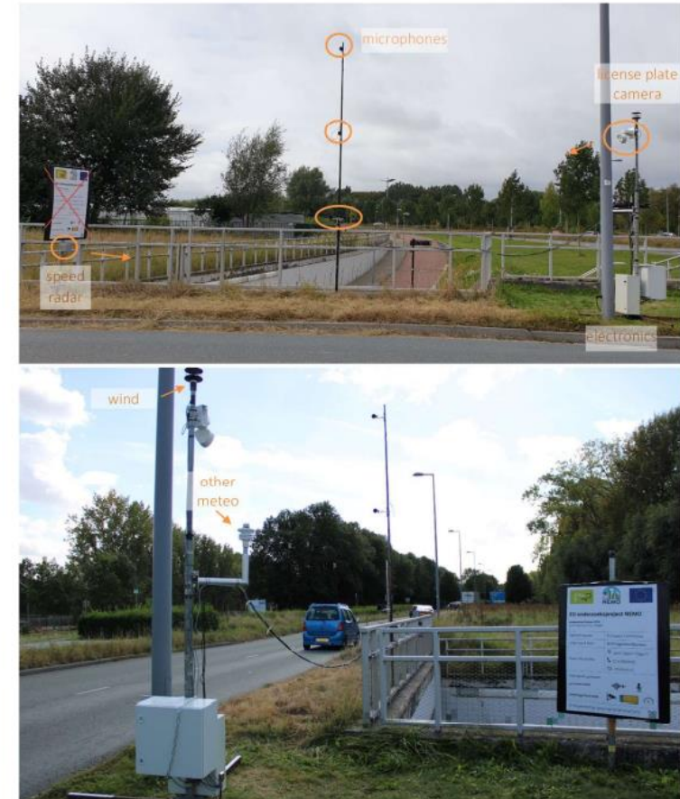
Figure 1: The NEMO noise-RSD measurement setup in Rotterdam, October 2021
